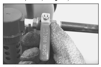
Figure 8. Tank air supply valve, closed.
